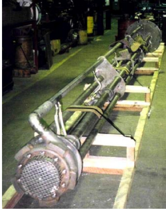
Figure 3-3. Long-shafted pump (Barth 2009).
