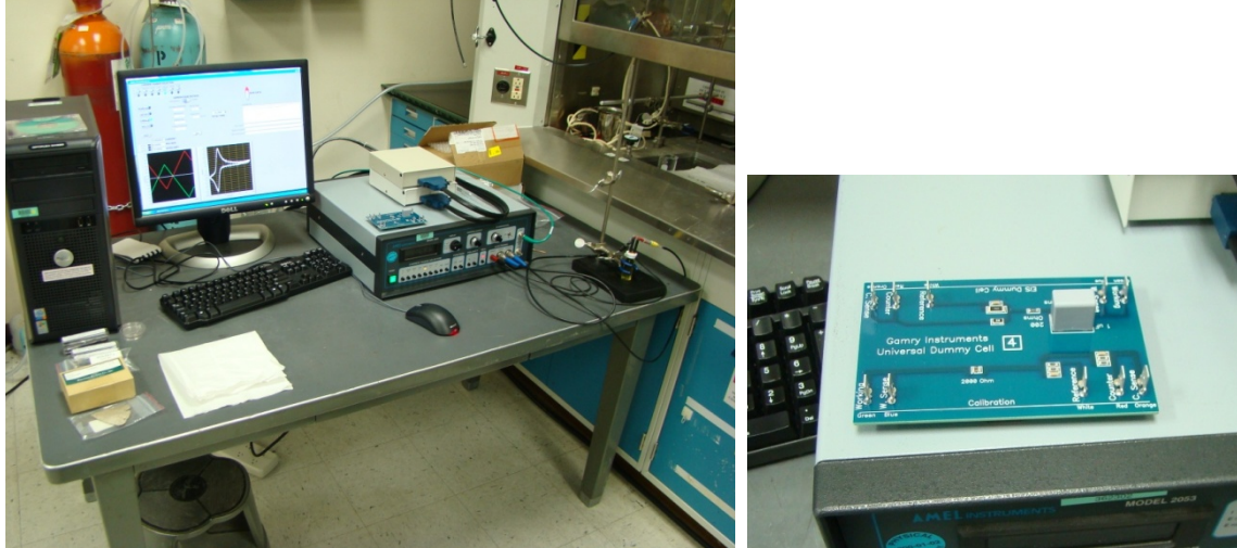
Figure 7-2. AMEL potentiostat with Labview interface (left) and dummy cell (right).
