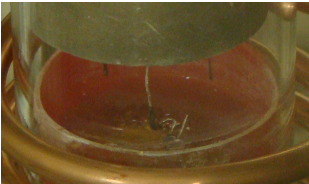
Figure 7-7. Platinum electrodes during operation: the counter electrode bent shape is visible.
